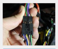
Connect the OEM connector to the supplied CAN IN/OUT
