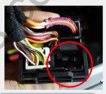
Reconnect the supplied cable where the black connector was removed.
